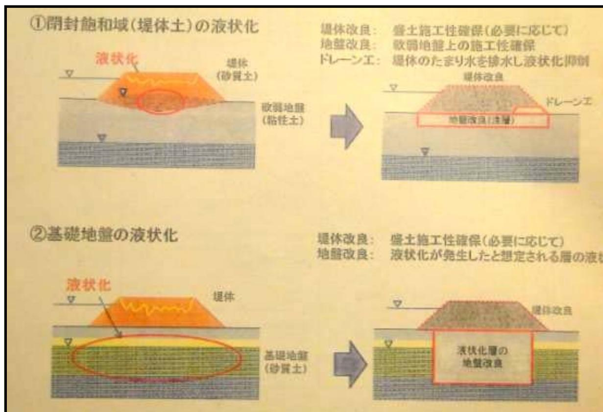
Figure 13: Drawing Depicting Permanent Repair Approach Using Foundation Treatment for Levees Seriously Damaged by Liquefaction (from MLIT, 2011)
