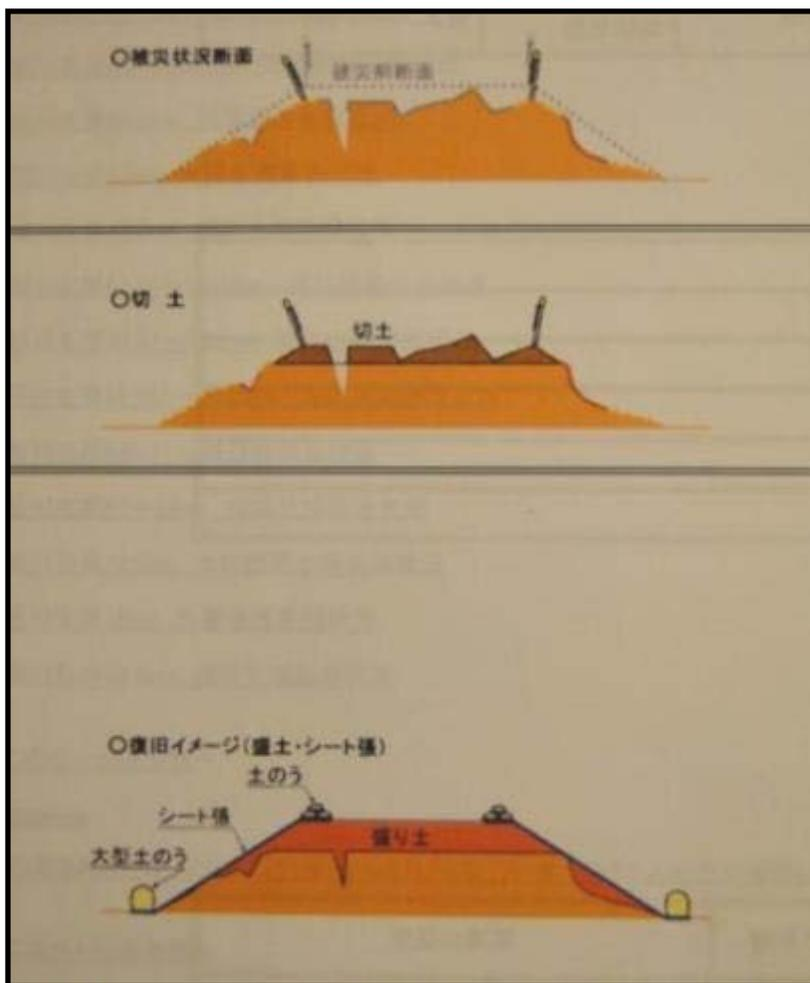
Figure10: Drawings Depicting Conceptual Approach for Interim Levee Repairs
