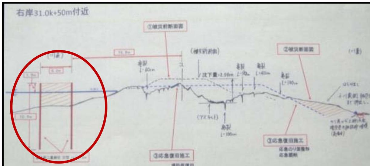
Figure 11: Drawing Depicting Sheetpile Interim Repair for Liquefaction-Related Damage on Abukuma River Levee at River Kilometer 31+50 (from MLIT, 2011)
